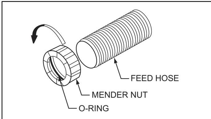
2. Place mender nut on Legend® II Swivel Mast. Connect the open end of the Feed Hose to the top of the Legend® II Swivel Mast and secure with the mender nut. The arch of the Feed Hose should align in the same direction as the Swivel Mast, there should be no twist in the Feed Hose after connection. (See illustration below.)
