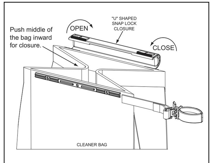
To close, push the middle of bag inward, as shown, and bring the edges together to make them stack like an accordion. Swing the "U" shaped snap lock closure back to the closing position.
