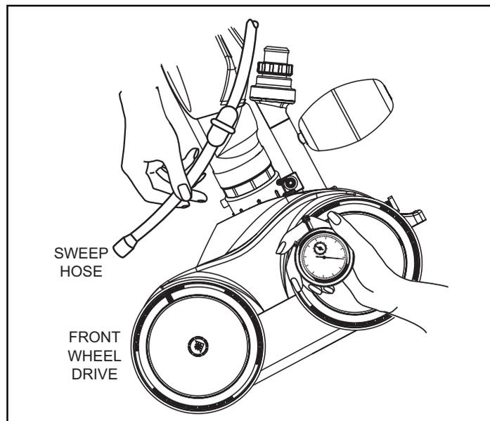
Mark the front drive Tire/Wheel with a marker, or use the Logo located on the side of tire as a marker to count the rotations of the wheel per minute.
