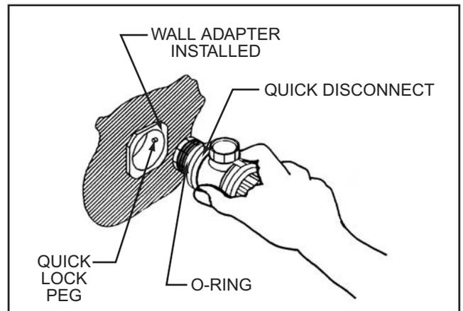
5. Take the Wall Fitting and Twist Lock the Wall Fitting into the Wall Adapter 1/4 turn; to a snug fit. Once the Wall Adapter is secure you can now twist lock and unlock to remove Wall Fitting with ease from the Wall Adapter.
