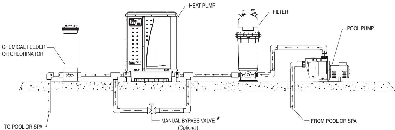
To Pool < Chlorinator or Chemical Feeder < Heat Pump < Filter < Pump < Skimmer and Main Drain < From Pool
