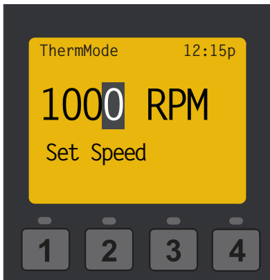
Setting the Thermal Mode Pump Speed
