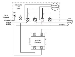
AutoSet Contactor to Mechanical Timer Wiring Example
