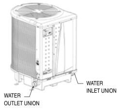
Heat Pump Water Connections
