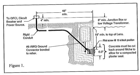
Some of the requirements of the National Electrical Code which the pool's electrical system must meet are as follows:
