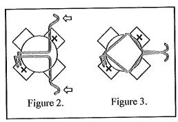
H. Replace the light assembly into the niche and tighten the special pilot screw.
