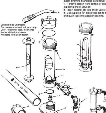
YOU MAY SUBSTITUTE BROMINE TABLETS OR STICKS FOR TRICHLOR IN THIS FEEDER. DO NOT MIX.
