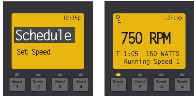
**Note:** The pump will not run the scheduled speeds until the **Start/Stop** button is pressed (LED on) to place the pump in Schedule mode.
