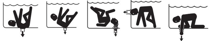
THIS PUMP PRODUCES HIGH LEVELS OF SUCTION AND CREATES A STRONG VACUUM AT THE MAIN DRAIN AT THE BOTTOM OF THE BODY OF WATER. THIS SUCTION IS SO STRONG THAT IT CAN TRAP ADULTS OR CHILDREN UNDER WATER IF THEY COME IN CLOSE PROXIMITY TO A DRAIN OR A LOOSE OR BROKEN DRAIN COVER OR GRATE.
