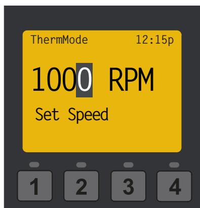
Setting the Thermal Mode Pump Speed
